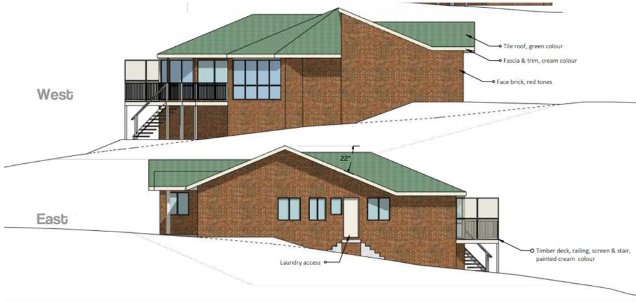
Figure 8: Existing side elevations
